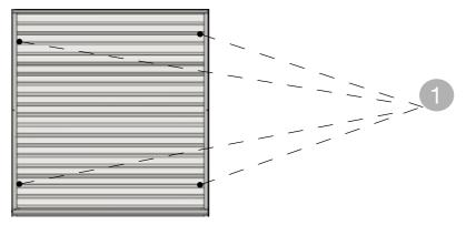
Then, install the louvre frame with the drip edge facing downward.
